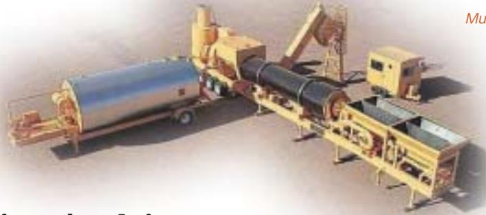
*Much Asphalt has taken delivery of its first, highly mobile Nomad hot mix asphalt plant valued at around R3-million. Imported from the United States, the plant is made up of four portable trailer mounted units and has the capacity to produce 120 tons of hot mix asphalt per hour.*
