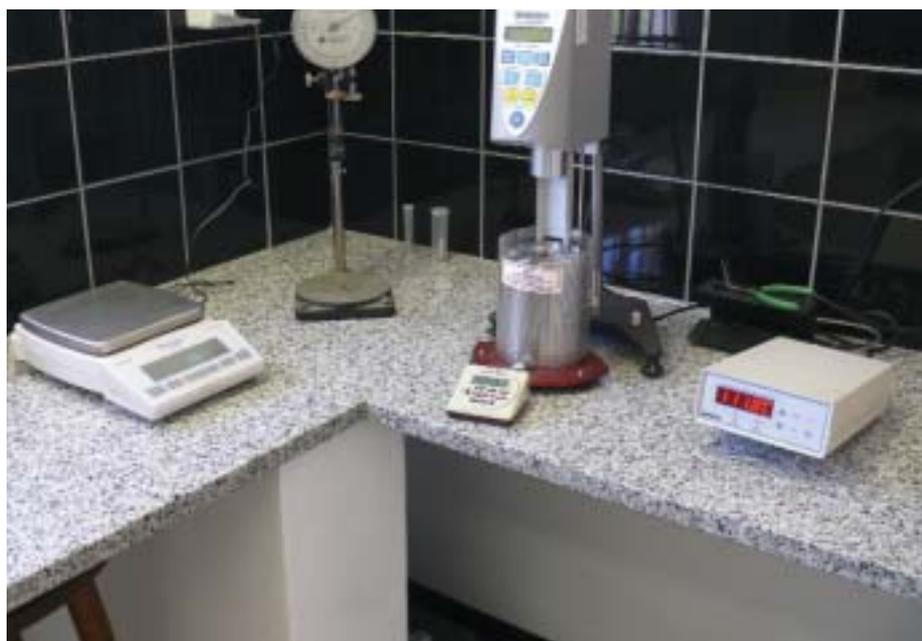
*New bitumen testing equipment (from left) balance, penetrometer and the Brookfield Viscometer with temperature controller.*
