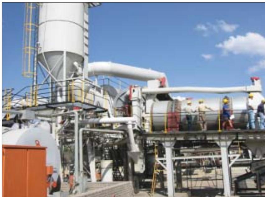
*The unique locally designed and built twin-drum mix plant at Much Asphalt Roodepoort.*
