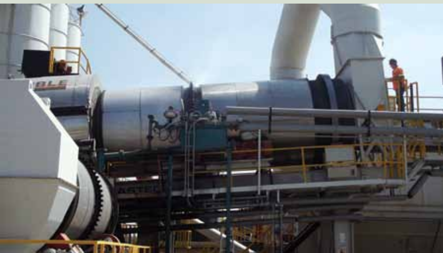
Benoni 2 plant foaming 55% BTB mix.
