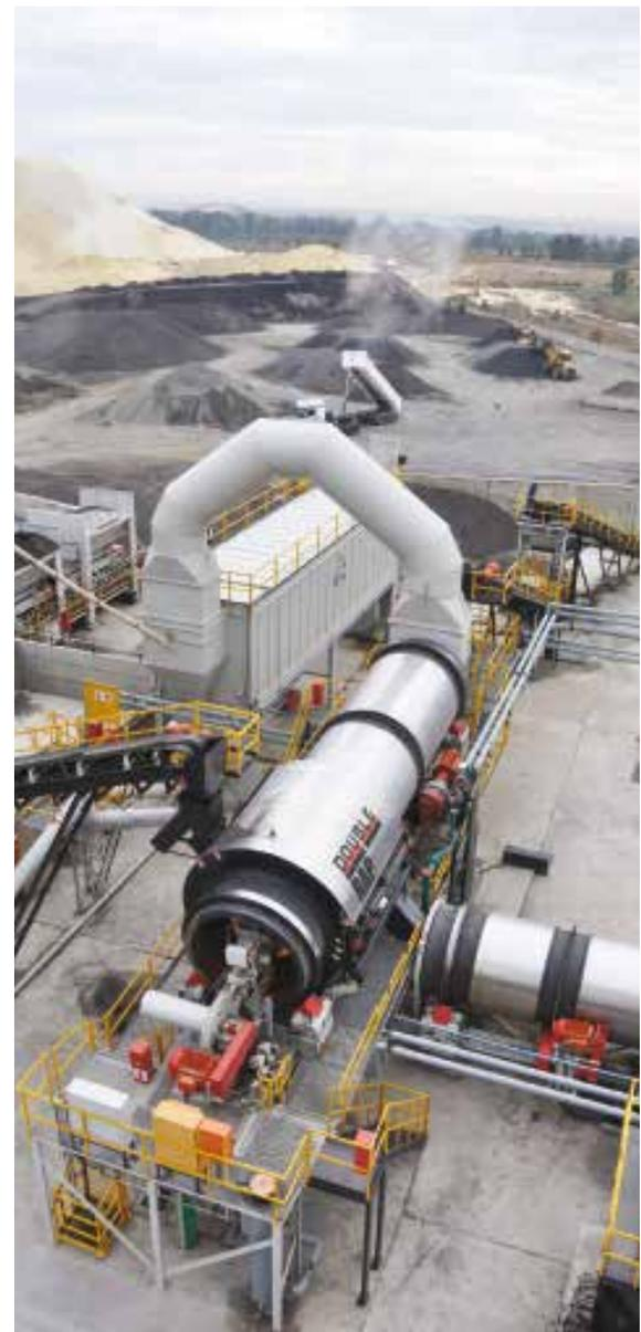
*Double barrel RA twin drum with foaming capabilities
